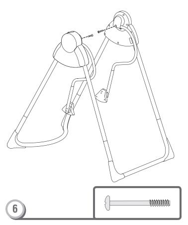
• Insert a #4 x 3,18 cm screw into each hub and tighten.
